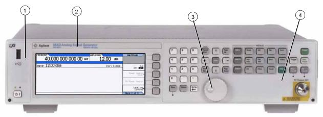
Figure 2-15 N5182A Front Panel View
